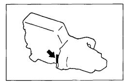
The number is punched on the cylinder block.
