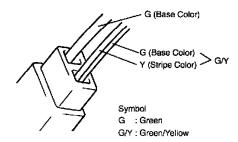
There are two types of wire color: one-color type and 2-color type(with a stripe). In case of 2-color type, the first alphabet ("G" of the example in the figure at the left) represents the basic color(color of wire insulation) and the next alphabet ("Y" of the example) represents the color of stripe.
