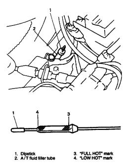
4. Lower vehicle and fill proper amount of an equivalent of DEXRON(R)III.
