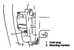
Install drain plug. Tightening Torque
