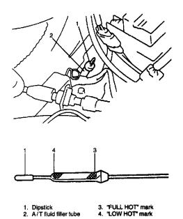
Pull out dipstick again and check fluid level indicated on it. Fluid level should be between FULL HOT and LOW HOT. If it is below LOW HOT, and an equivalent of DEXRON(R)III up to FULL HOT. Fluid specification: An equivalent of DEXRON(R)III
