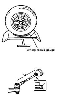
When tie rod or tie rod end was replaced, check toe and then also steering angle with turning radius gauge. If steering angle is not correct, check if right and left tie rods are equal in length ("A").
