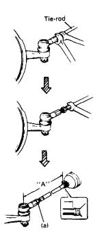
Toe is adjusted by changing the tie rod length. Loosen right and left tie rod end lock nuts first and then rotate right and left tie rods by the same amount to align toe-in to specification. In this adjustment, right and left tie rods should become equal in length ("A" in figure shown).
