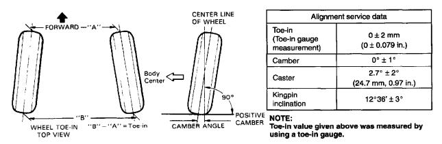
Front alignment refers to the angular relationship between the front wheels, the front suspension attaching parts and the ground. Generally, the only adjustment required for front alignment is toe setting.
