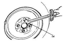
Tightening Torque for wheel nuts (a): 85 Nm (8.5 kg-m, 61.5 ft. lbs.)
