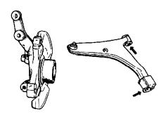
SUSPENSION ARM/ STEERING KNUCKLE CHECK Inspect for cracks, deformation or damage.
