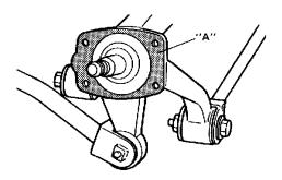
3. Apply water tight sealant to mating surfaces of brake back plate and rear knuckle. "A": Sealant 99000-31090
