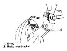
2. Remove E-ring securing brake hose.
