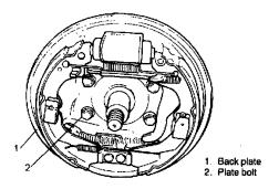
5. Remove brake back plate from knuckle.
