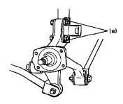
2. Tighten strut bracket bolts and nuts to specified torque. Tightening Torque (a): 90 Nm (9.0 kg-m, 65.0 ft. lbs.)
