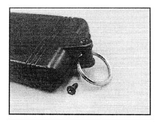
To open the case, first remove the small phillips screw. Then gently pry the case apart.
