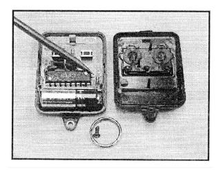
With the case apart, locate the Zener diode as indicated by the pointer in the picture to the right.
