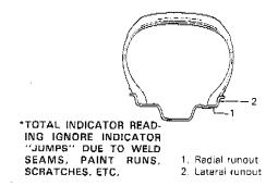
Take measurements of both lateral runout and radial runout at both inside and outside of the rim flange. With the dial indicator set in place securely, turn the wheel one full revolution slowly and record every reading of the indicator.
