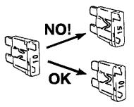
^ When replacing a fuse, make sure to use a fuse of the specified capacity. Use of a fuse with a larger capacity will cause a damage to the electrical parts and a fire.
