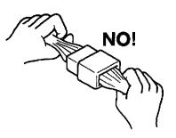
^ When disconnecting connectors, never pull the wiring harnesses. Unlock the connector lock first and then pull them apart by holding connectors themselves.
