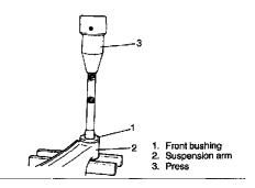
8. Cut off flange of front bushing and then push out front bushing by using hydraulic press.
