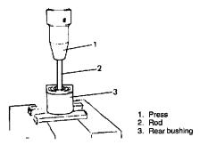
7. Remove rear bushing by using hydraulic press.
