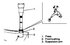
1. Install front bushing. Before installing bushing, apply soap water on its circumference to facilitate installation. When installed, bush should be equal on the right and left of arm as shown.
